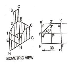
8. A vertical square prism, base 40 mm side, is completely penetrated by a horizontal square prism, base 30 mm side, so that their axes intersect. The axis of the horizontal prism is parallel to the V.P., while the faces of the two prisms are equally inclined to the V.P. Draw the projections of the solids, showing lines of intersection. (Assume suitable lengths for the prisms).
